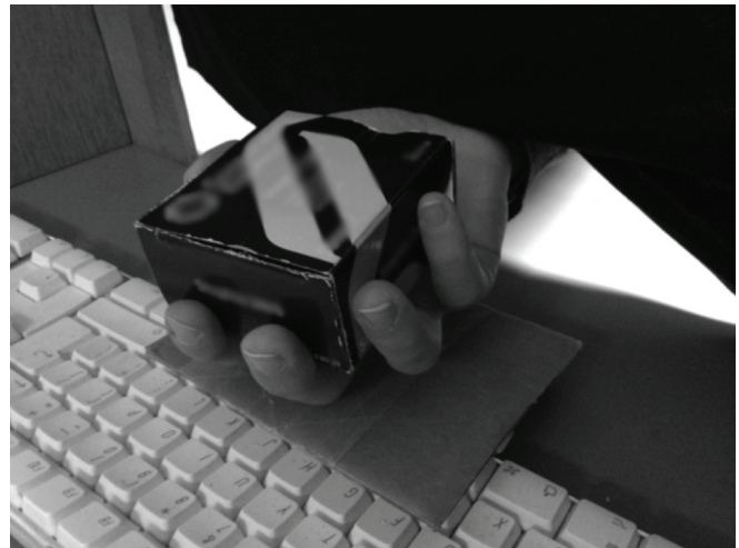
Figure 1. A participant holding the box with the hand still resting on the platform mounted on the keyboard. Lifting the hand triggered the start of a trial. The hand was occluded from view by a curtain.
