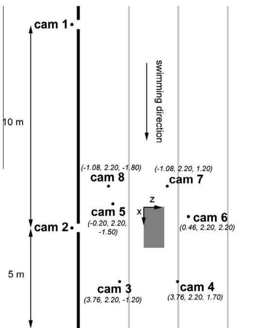
**Fig. 3.** Positioning of the two cameras (cam 1 and 2) in the wall and the six cameras (cam 3–8) used for 3D reconstruction around the calibration volume (grey square). Camera coordinates are given in meters relative to the upper left corner of the calibration volume.
