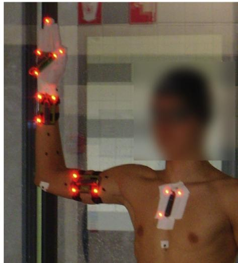
Fig. 2. The rigid body with three LEDs (A–C) mounted on it.
