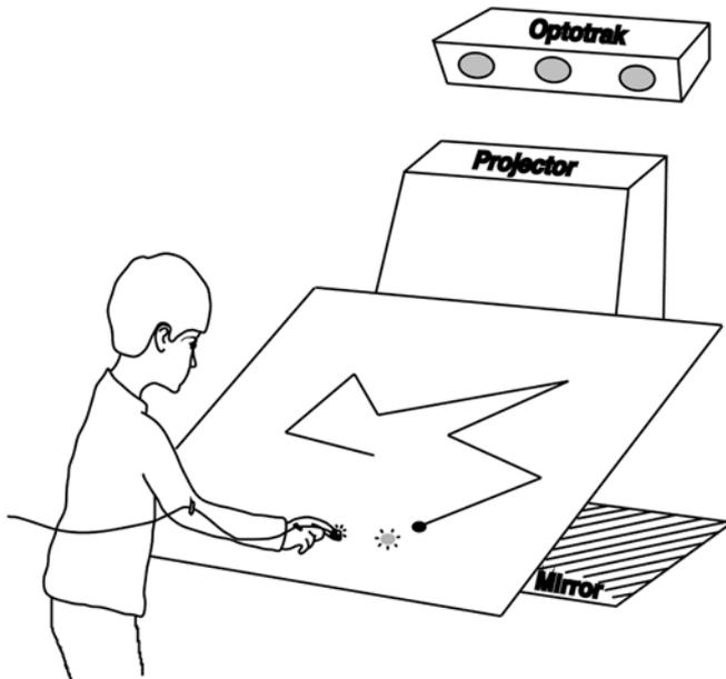
**Fig. 1** Schematic drawing of the set-up. A flash (grey disk) is just being presented to the subject. The connected line segments indicate a piece of the path that the pursuit disk (black disk) followed; the subject never saw this. In this case the flash is presented ahead of the pursuit target
